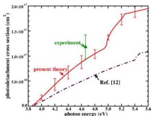
Here the Quantemol interface has been used to compare experimental and theoretical photodetachment cross sections. The R-matrix code was used for the  $\text{CN}$  and  $\text{CN}^-$  molecules by Khamesian et al, 2016 .
