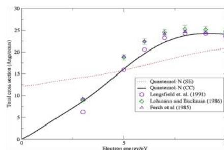
Total cross-sections of  $\text{CH}_4$ . Here the Quantemol-N results (black & red lines) are shown with theory (Lengsfeld et al., circles) and experiment (Lohmann & Buckham, diamonds, Ferch et al., triangles).
