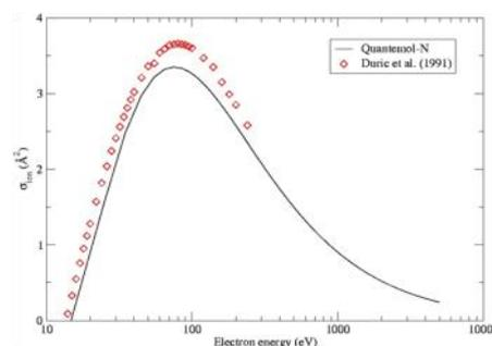
BEB ionisation cross-section of  $\text{CH}_4$ . Here the Quantemol-N data is compared with experimental data (Duric et al., red diamonds).
