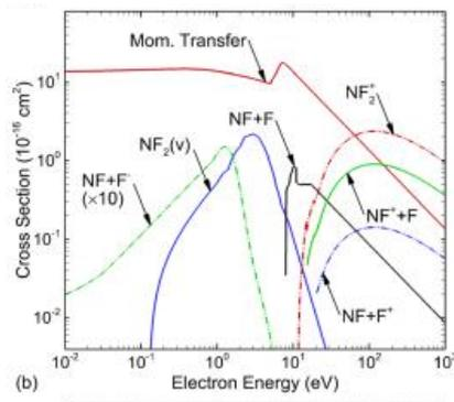
Cross sections for electron impact reactions of  $\text{NF}_2$  using the *ab initio* molecular R-matrix method. Huang et al, 2017.
