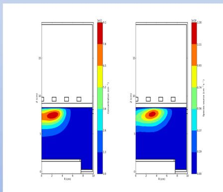
Figure 1. Electron density (left) and atomic fluorine production rate (right) in an SF<sub>6</sub> discharge at 75 mTorr and 800 W.
