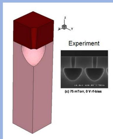
Figure 4. Resulting etch profile of silicon by chemical etching and comparison to experimental results [3].
