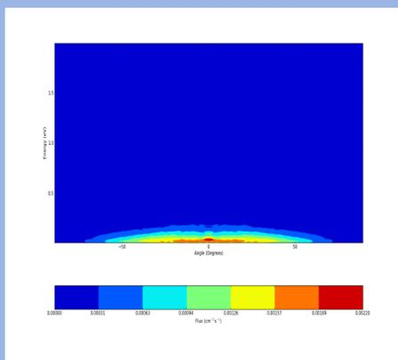
Figure 3. Energy and angular distribution functions of atomic F at the wafer in an SF<sub>6</sub> discharge at 75 mTorr and 800 W.
